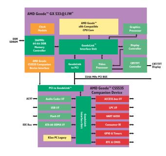
Optimized for low-power applications such as set-top boxes, personal access devices, thin-client applications and other products that combine low power requirements with small form factors, the AMD Geode<sup>™</sup> GX 533@I.IW processor provides the maximum mix of performance, power and size. The AMD Geode CS5535 companion device enables fast design-to-market cycles.
